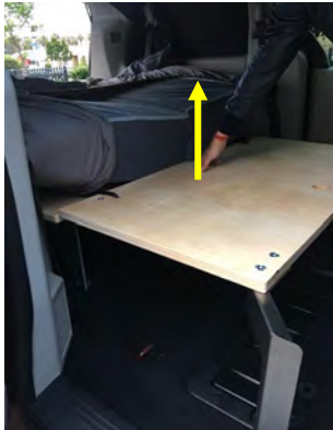
3. Using the hole at the center back of the panel, lift the panel and tuck it between the mattress and the middle panel.
