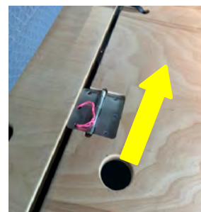
Check position – pull upwards lightly - the front board cannot be lifted up or moved backwards when properly locked.
