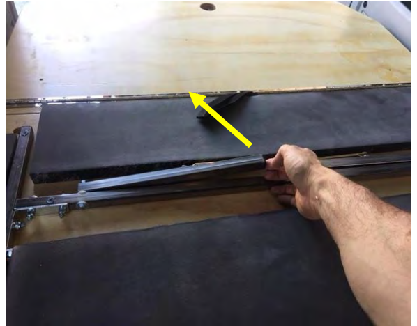
2. Lift support legs on front panel
