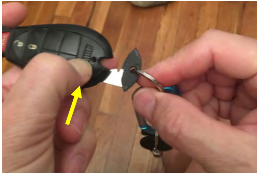
1. Slide the latch to the right (left thumb shown here sliding the latch).
