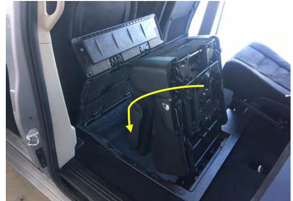
6. Push seat in to the cavity.
