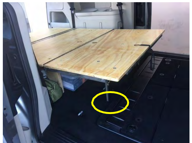
6. Make sure legs rest on the carpet just behind the plastic cover.
