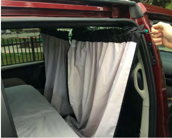
1. The curtain is threaded on a bungee cord with a metal hook in the middle.
