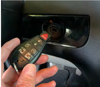
1. Insert the key fob to the switch as shown
