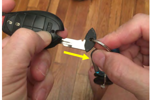
2. While keeping the latch pushed to the right, pull on the key ring to remove the key.
