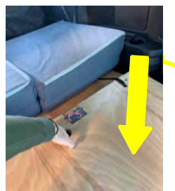
2. Push down when the back edge of the front board passed the edge of the middle board
