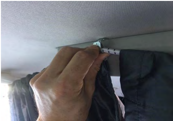
3. Insert the hook between the roof and the roof console (2018 Caravan console shown)
